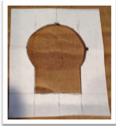
Figure 1: Paper template to position hole for element.
