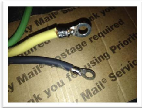
Figure 5: Ring terminals soldered onto the ends of the power cable.
