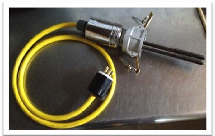
Figure 6: Final assembly of the Cam & Groove electric heater element.
