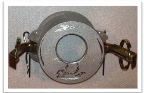
Figure 2: Cam & Groove cap coupling with 1-1/4" hole drilled for element.
