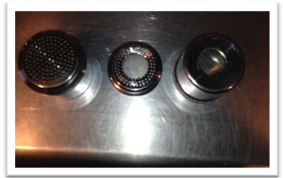
Figure 4: Stainless steel shaker with holes drilled in cap and bottom of shaker.
