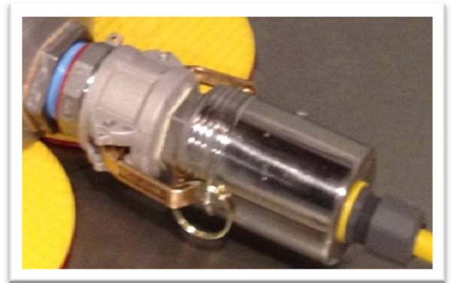
Figure 8: Cam & Groove electric heater element attached to kettle.
