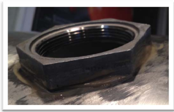
Figure 7: Locknut glued to exterior of kettle.
