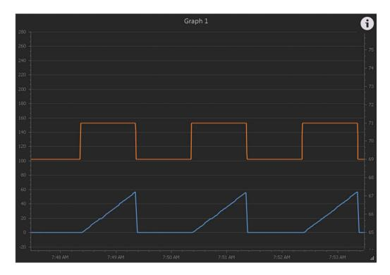
With a large increase in the Derivative, we should not see such rapid changes in direction, D of this PID is not working as expected... we should be able to get a sine wave, but we cannot even change the downward slope...
