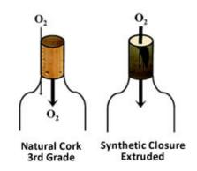
Results for the natural cork showed diffusion of oxygen at a slow but continuous rate over the first 12 months of storage and in very tiny amounts through the cork–glass interface in the 12 months thereafter. Results for were similar under all test packages indicating that oxygen originated inside the cork and was transmitted by diffusion.
