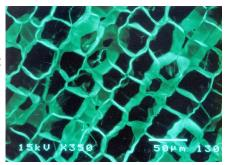
Natural cork consists of millions of tiny "cells" – 40 million cells fit in one cubic centimeter. Each cell is filled with air, and that air provides a small dose of oxygen for each bottle.
