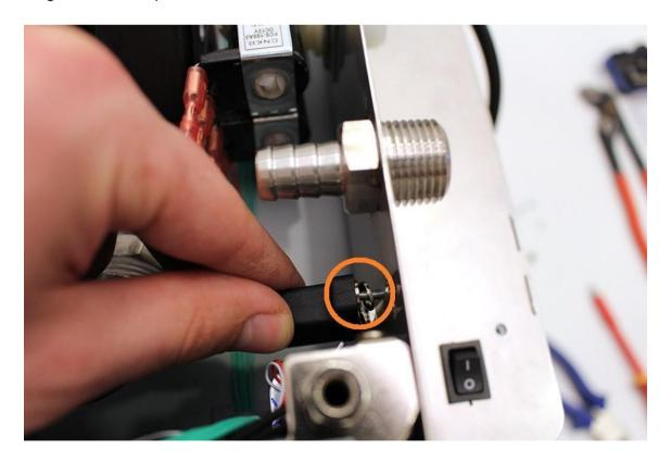
Loosen the indicated hose clamp and remove the high pressure hose from the fitting.
