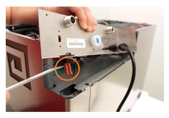
Remove the cables from the cable clips.
