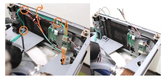
Remove the cables from the indicated cable clips.
