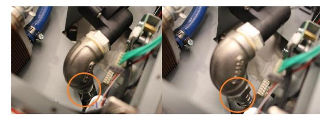
Bend the pump holder sheetmetal carefully in order to remove the pump easier.
