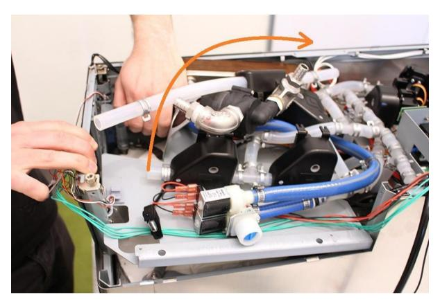
While lifting up the assembling sheetmetal, make sure not to damage the cables at the indicated areas.
