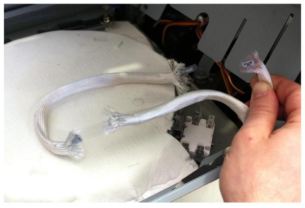
Carefully remove one side of the heat insulation.
