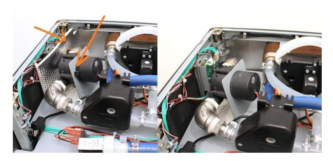
Pull off the pipe clamp from the encircled fitting. Pull off the silicone hose from the fitting.
