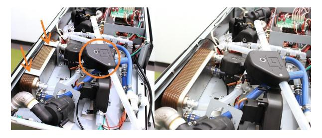
Unscrew the 4 indicated assembly plate screws.
