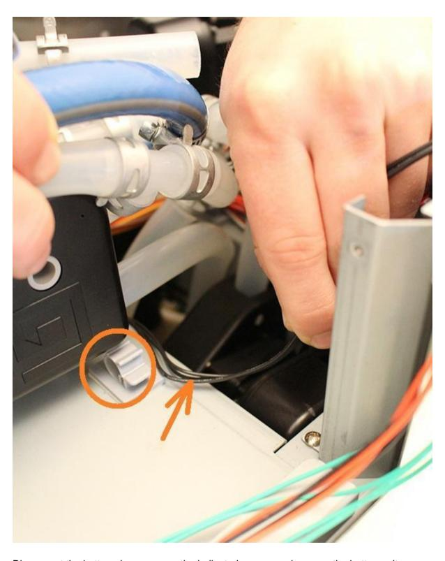
Disconnect the button plug, unscrew the indicated screws and remove the button unit.
