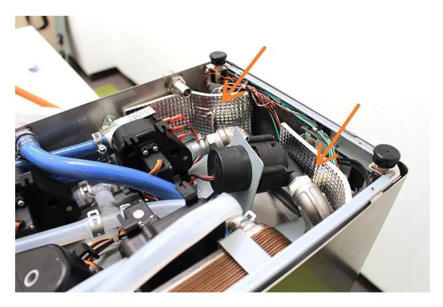
6. Make sure that the wort outlet hose clamp is in the proper angle. Otherwise you cannot reassemble the lower sheetmetal.
