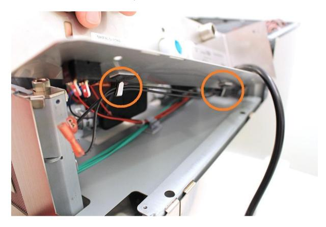
Pull off the high pressure valve from the sheetmetal. Pull off the sheetmetal on the power cable and put it on a safe place.
