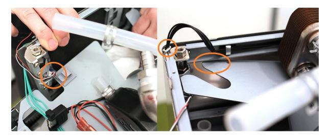
It's recommended to fix the assembling plate with a soft object as shown on the right picture.(It must be soft to avoid the scratches on the cover of the machine). Rotate the 4 indicated heat plate clamps to free the heatplate.
