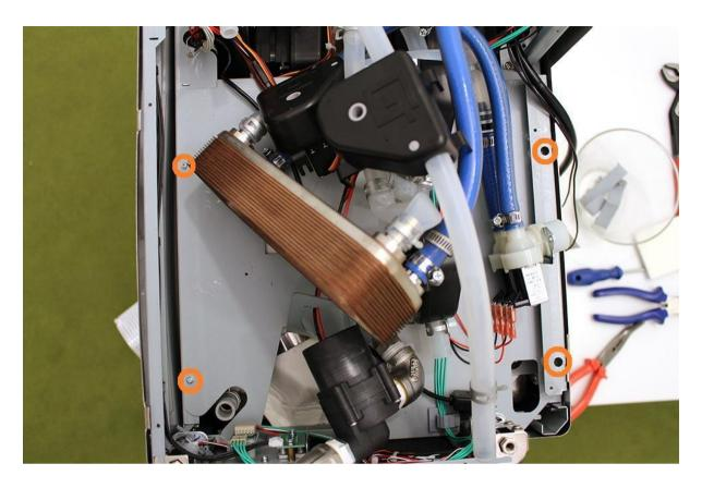
Disconnect the two indicated plugs, remove the cables from the indicated cable clips. Put the cables outside the machine in order to avoid the damage of the cables.
