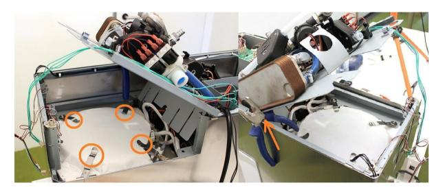
Remove the indicated heat plate cables.
