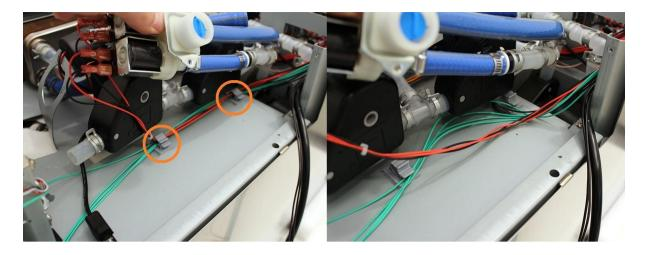
Remove the cables from the indicated cable clips. The right picture shows where to put the power and switch cords in order to avoid the damage of these cables.
