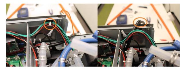
Remove the cables of the temperature sensor from the indicated cable clip. Avoid strain of this cable during further assembling.
