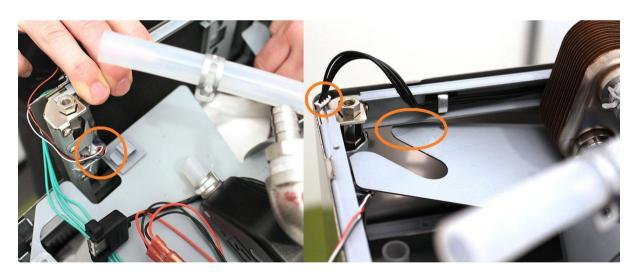
3. Be careful with the silicone flange around the button while reassembling the button!
