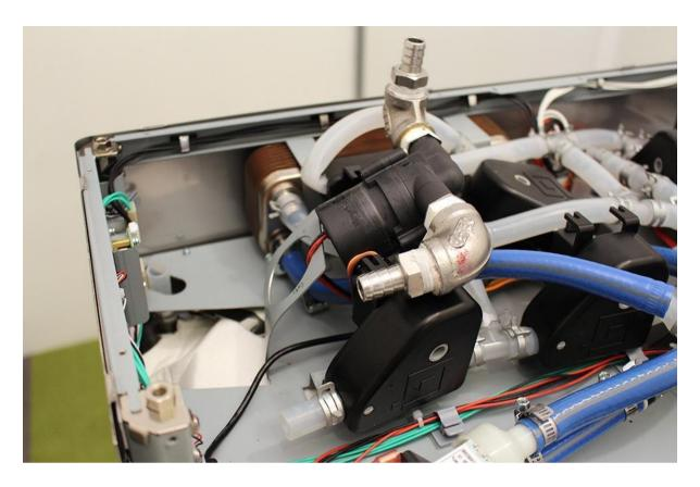
Remove the indexed valve (see at: "Remove the wort outlet valve"). Remove the heat exchanger holder clamps.
