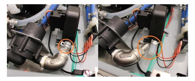
While you loosen the indicated hose clamp, you can pull off the pump from the silicone tube by rotating the pump around its axis.
