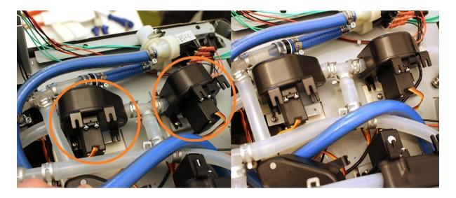
Lift the assembly plate carefully. Make sure not to damage the cables by the sheetmetal.
