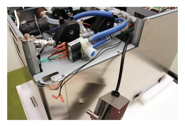
Remove the indicated heat insulation and remove the indicated cable tie.
