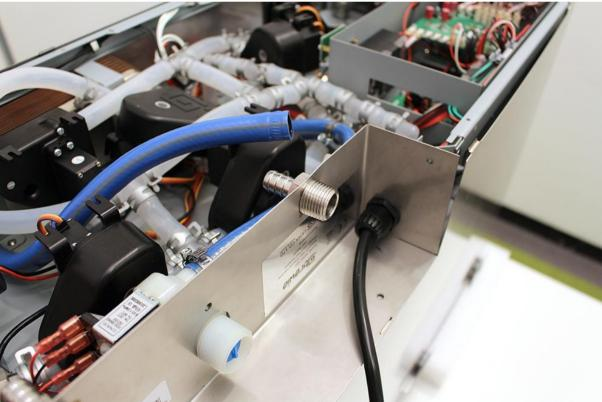
Lift the sheetmetal part carefully and disconnect the indicated plugs with a screwdriver.
