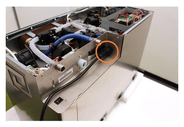
Remove the wort outlet hose clamp, pull off the wort outlet silicone tube and unscrew the indicated screws.
