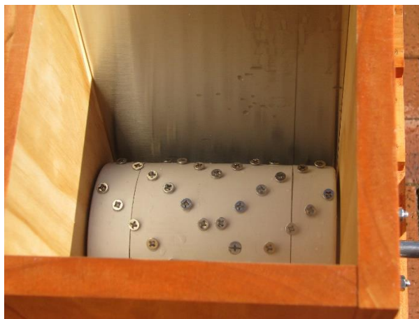
Paper Drilling Pattern wrapped around the drum, then screws in place
