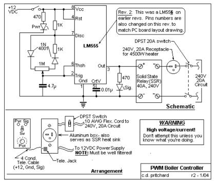
(The schematic in the above drawing was revised on 1/05 to show a LM555 instead of a LM556 so that it agrees with the PC baord layout below)
