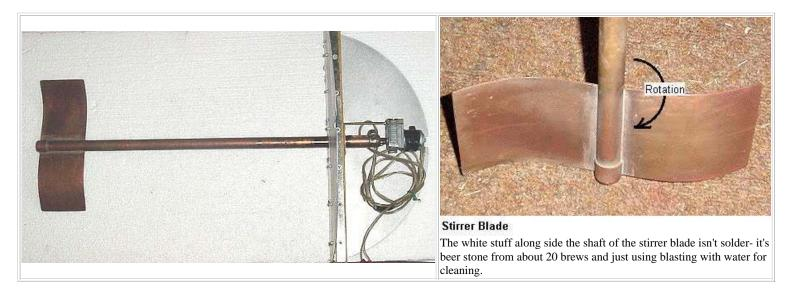
A stirrer is *NOT* needed to prevent scorching, but, when used during the boil, it does appreciably increase hop utilization. Where it's of immense benefit is when cooling the wort- it GREATLY shortens the amount of time required since the wort is being moved over the surfaces of the immersion chiller thereby increasing heat transfer.
