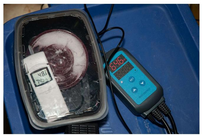
As you can see above, I set up the saturated salt in a small plastic box along with both the Ecowitt and the probe for the Inkbird and it was readily apparent the Inkbird was reading way low.
