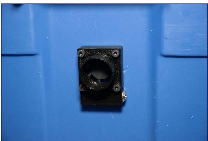
Above are the 3d printed pieces hold the dc power connector for the fan and the filter. I gave up trying to make the "ears" to hold the filter on the snoot and settled for simply using hot melt glue to hold the filter on.
