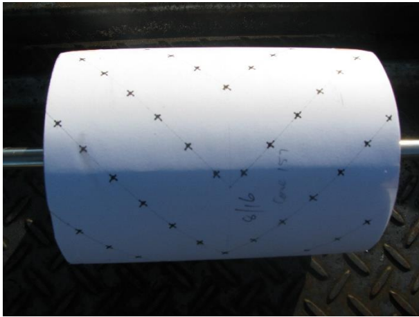
Paper Drilling Pattern wrapped around the drum, then screws in place
