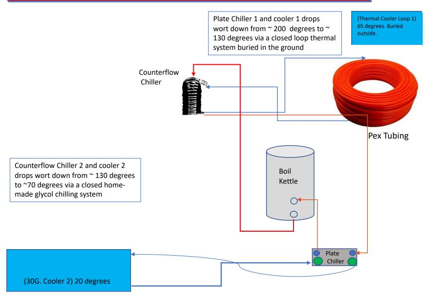
Note: Wort is in series with the chillers utilizing a closed recirculation method. Pumps are not illustrated.
