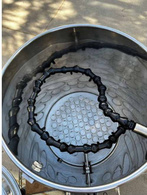
Mash Tun with false bottom and adjustable sparge arm.
