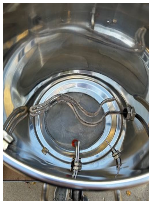
Boil Kettle with Hop Stopper screen and 220v heating coil.
