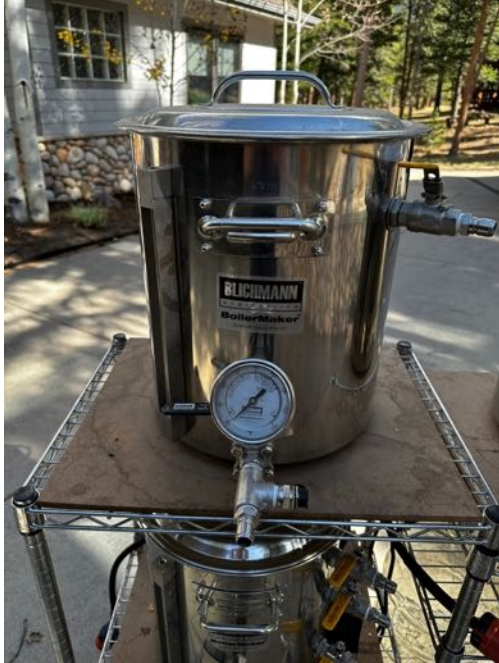
Mash Tun with false bottom and adjustable sparge arm.
