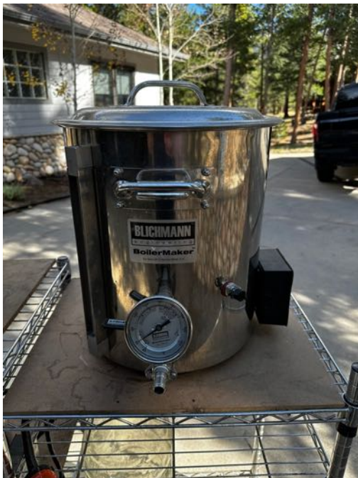
Boil Kettle with Hop Stopper screen and 220v heating coil.
