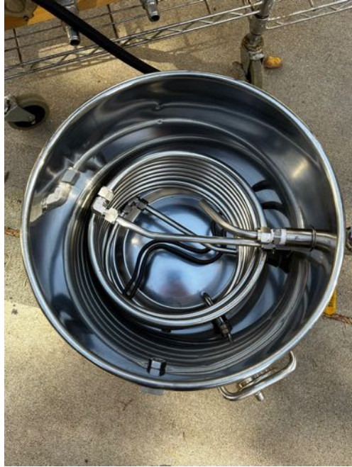
Hot Liquor Tun with stainless coil and 220v heating coil.
