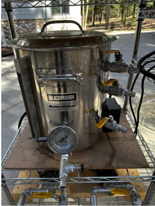
Hot Liquor Tun with stainless coil and 220v heating coil.
